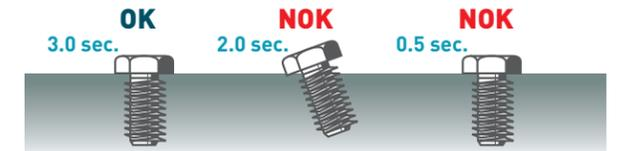
Finished with 3.0 sec. rundown time Finished with 2.0 sec. rundown time due to cross thread Finished with 0.5 sec. rundown time due to re-tightening
